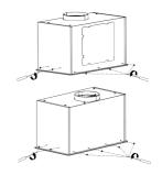
Disconnect the two plugs from the switch cable and the lamp cable, remove the cover panel and place it on a smooth, level surface.
